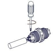
5) Insert connectors to hole of chassis then lock the parts.
