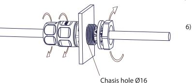
Chassis Max Thickness 3,5 mm
