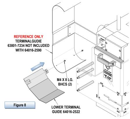
**NOTE**: Clearance holes may need to be drilled into the existing terminal guide on some older TM3000 presses.
