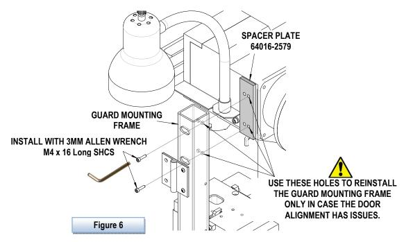
7. Important Locate the new spacer plate (64016-2579) <u>BETWEEN</u> the guard mounting frame and the press. **Note:** Make sure to use the <u>RIGHT SIDE</u> set of mounting holes. See Figure 6.
