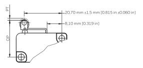
NOTE: These dimensions apply for the "A" lever position. For the "B" lever position, please add 5,8 mm [0.224 in].
