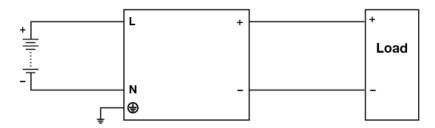
Fig. 6 DC Input Operation Connection Diagram
