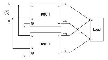
Fig. 5 Parallel Operation Connection Diagram
