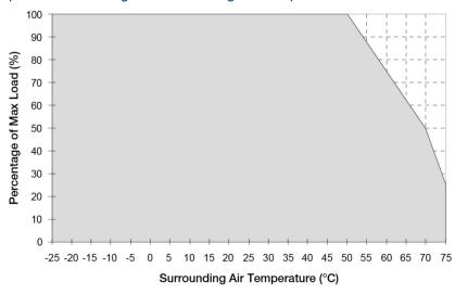
Fig. 1 De-rating for Vertical Mounting Orientation
