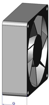
For the article definition you need the fan size (size B), the flange thickness (size G/ see picture left) and also the panel thickness.
