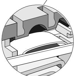
Two-piece spring and carrier mechanism gives extra long electrical and mechanical life.
