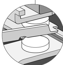
High contact reliability - optimum reliability due to high contact force
