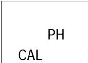
6) Press the " ▲ Button " ( 3-5, Fig. 1 ) or " ▼ Button " ( 3-6, Fig. 1 ) once in sequence to select the following screen.
