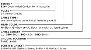
${\bf 3}{=}{\rm White}$  Silicone Profile Gasket & Screw,  ${\bf 4}{=}{\rm White}$  Silicone Flat Gasket & Screw  ${\bf P}{=}{\rm NBR}$  Integrated Gasket Assembled + IP67 Screw
