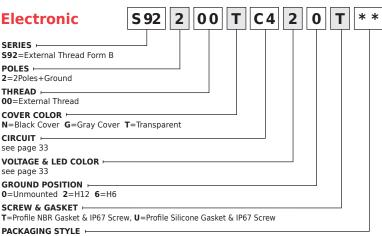
no digit=Single Bag Unmounted, SN=Bulk Pack Mounted, CN=Bulk Pack Unmounted
