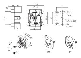
DIN Bases are provided in kit with fixing screw and gasket where required. The range covers the most important and common applications.
