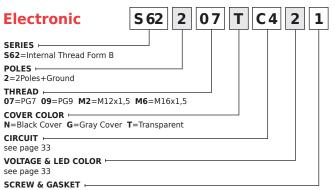
1=Profile NBR Gasket & Screw, 2=Flat NBR Gasket & Screw 3=White Silicone Profile Gasket & Screw, 4=White Silicone Flat Gasket & Screw
