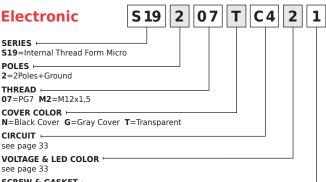
1=Profile NBR Gasket & Screw, 2=Flat NBR Gasket & Screw 3=White Silicone Profile Gasket & Screw, 4=White Silicone Flat Gasket & Screw
