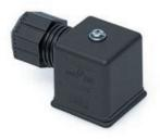
IP67 rated DIN valve connectors with improved strain relief. Cable retention force increased by up to 20% over internal nut styles. Enlarged cable range that covers the PG9 and PG11 internal thread connector cable range. Conforms to EN 175301-803.
