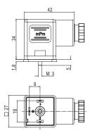
Note: UL listed part number identified by adding suffix SA at the end of the nomenclature in conjunction with UL material (W for black and T for transparent) e.g. C28200W2RSN<mark>S</mark>A
